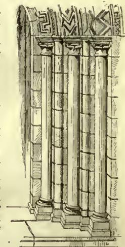
an upright timber at the side of an aperture, as of a doorway, window, fireplace, etc.
